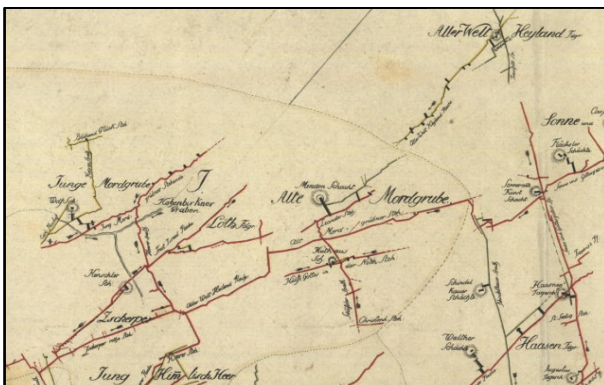
Fig. 8: The galleries of the Neuen Tiefen Fürsten Stolln inside the mining field of the Alten Mordgrube (plan section late 18 th century).
